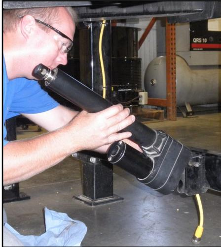
When removing the actuator (03-17-0104) from the box, ensure that you do not allow the shaft to rotate. The actuator was installed and tested at the factory so the shaft is in the correct position before it was disassembled prior to shipping.
