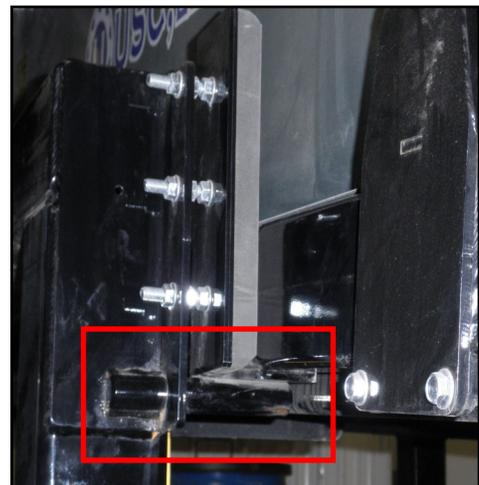
**STEP C:** Lower the drum slowly until the drum frame is resting on the dead stop pins on both sides of the treater frame.
