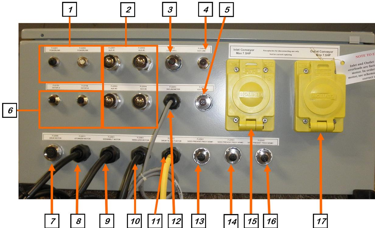
1. Connect a cable with four pin connector to one of the three Powerlink connectors on the MCP. Connect the other end to the Powerlink connector on the closest control panel. Repeat this process until all control panels are connected. It may be MCP to Treater to Tri-Flo® to Bin Site panel. The order or number of devices is not important. It is important that all panel are connected. All pump stand control panels will need to connected in a similar configuration.
