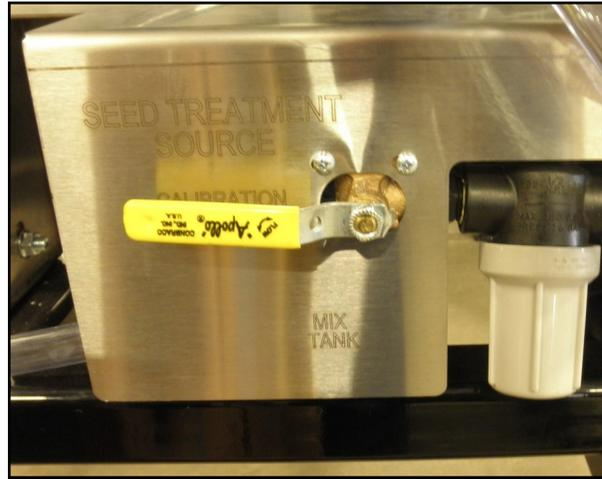
*Pump #1 Drawing from bottom of Calibration Tube*
