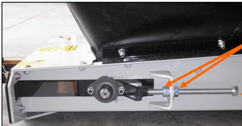
*Loosen the jam nuts before adjusting the bearing position bolt*
