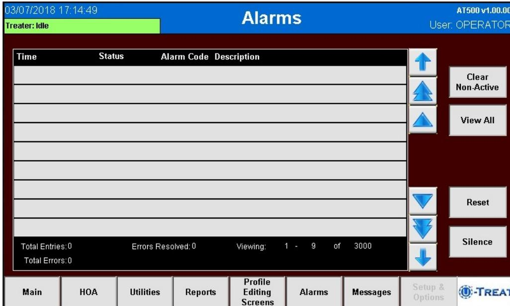
**1. CLEAR NON-ACTIVE:** The alarm status will change to Acknowledged once an alarm condition has been resolved and the Reset button has cleared the alarm. Pressing this button will clear all alarms with the status of acknowledged.
