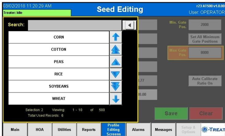
**1A. MINIMUM GATE POSITION:** Pressing this button brings up a keypad to enter a value for a minimum gate position for this individual seed profile.
