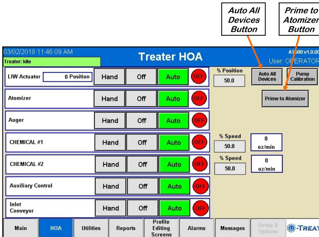
3. Return to the main screen and press the Start Setup button. Press the gray buttons to change the Recipe or Seed Type fields. Press Start to begin the run. The atomizer and auger will turn on. Open the manual gate on the box. When the proximity switch detects seed, a timer will count down the number of seconds the start delay was set for. When that time elapses, the slide gate will open.
