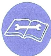
**Mandatory Read Manual Action Symbol.** (I.S.O. format) This symbol instructs personnel to read the Operators Manual before servicing or operating the equipment.
