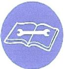
**Mandatory Read Manual Action Symbol.** (I.S.O. format) This symbol instructs personnel to read the Operators Manual before servicing or operating the equipment.
