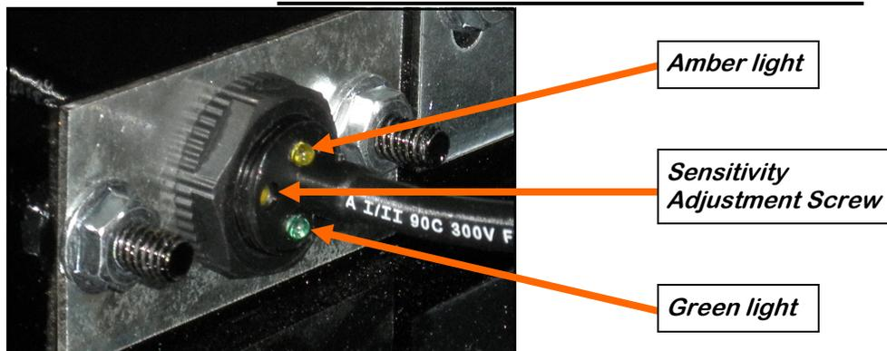
The proximity switches mounted in the extension ring and the seed wheel detect when seed is present.
