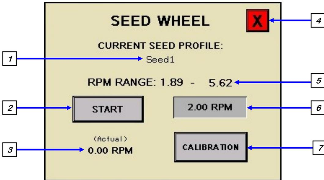
**1. CURRENT SEED PROFILE DISPLAY:** This displays the name of the seed type currently active in the system.
