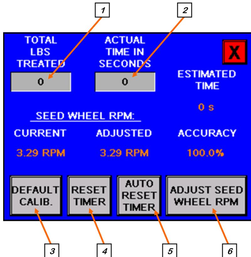
**1. TOTAL POUNDS TREATED:** Pressing this button will bring up a numeric keypad which allows the operator to manually input the amount that was treated.
