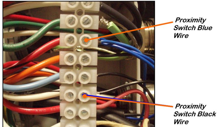
4. On LP seed treaters **ONLY**, the 4-pin cable coming out of the bottom of the seed wheel control panel wires into the seed treater panel.
