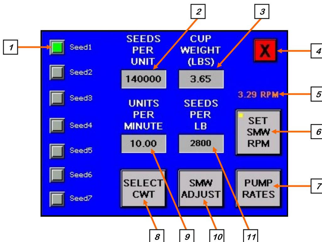
**1. SELECT SEED TYPE MODULE:** The operator can select between seven different pre-determined seed types. Press the name of the Seed Type and an alpha numeric keyboard will popup allowing the operator to change the name.
