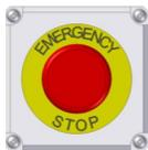
There are three Emergency Stop push buttons. There is one on the Main Control Panel, one on the Tri - Flo ® Control Panel and one on the Bin Site Control Panel. Actuators of emergency stop shall be colored RED. The background immediately around the device actuator shall be colored YELLOW. The actuator pushbutton-operated device shall be of the palm or mushroom head type.
