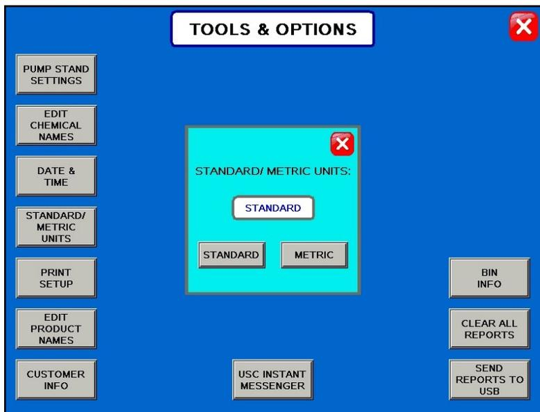
**5. PRINT SETUP:** Allows the operator to set up their personal company information which will be printed at the top of each report. Pressing the button will advance the operator to the screen below. The company information can be entered by selecting the blank space under each heading. The operator may also check the Auto Print box to print a report for a customer every time a report is generated as well as how many copies the customer requires.
