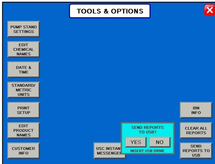
**11. USC INSTANT MESSENGER:** Pressing the button will advance the operator to the Instant Messenger screen. This allows the operator to communicate with the technical support staff. This option only functions if the operator has U-Connect light installed on their laptop or U-Connect Pro is connected to the control panel using a thin client to make the connection.
