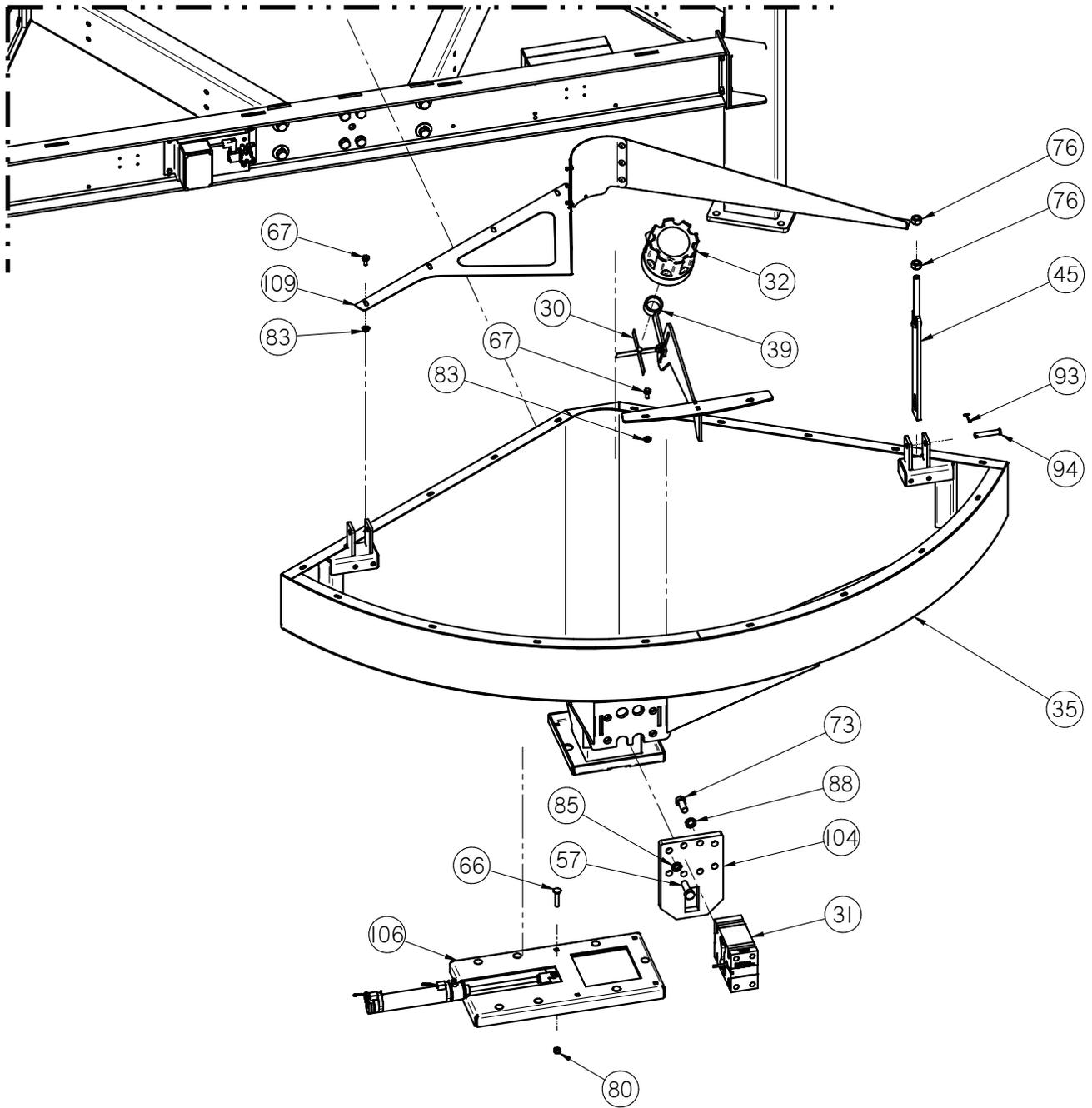
**TRI - FLO ® CONTROL PANEL - SCALE HEAD & PRINTER MOUNTING**
