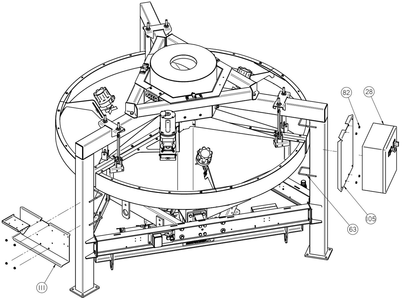
**TRI - FLO ® FORKLIFT POCKETS & SCALE CERTIFICATION WEIGHT BAR**
