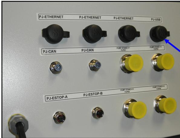
The USB port located on the bottom of the Main Control Panel allows the operator to download reports to a compact flash device.
