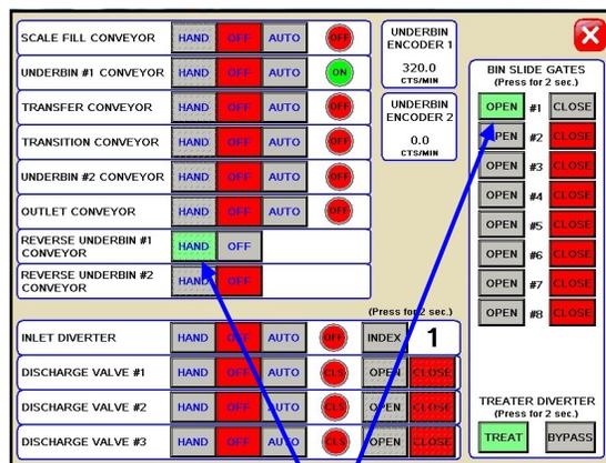
Press the “HAND” button and then place the bin slide gate to the “OPEN” position.
