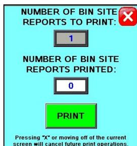
5. Once the data has been saved, the reports can be accessed later by pressing the REPORTS button on the UTILITIES screen. If you would like to erase the reports, press the SECURITY button under the UTILITIES screen to advance to the security screen. Enter the password **USC** and then press the TOOLS & OPTIONS button. From this screen press the CLEAR ALL REPORTS button. A confirmation window will appear allowing the operator to erase all saved reports.
