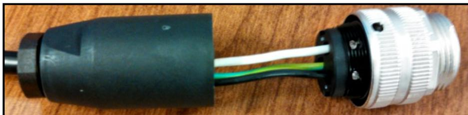
4. Line holes up so you can insert your small screwdriver into the part. Rotate the screwdriver side clockwise (while holding the black side) to reassemble. Tighten the black nut back down until the cord grip is tight on the insulation (page 18, top).
