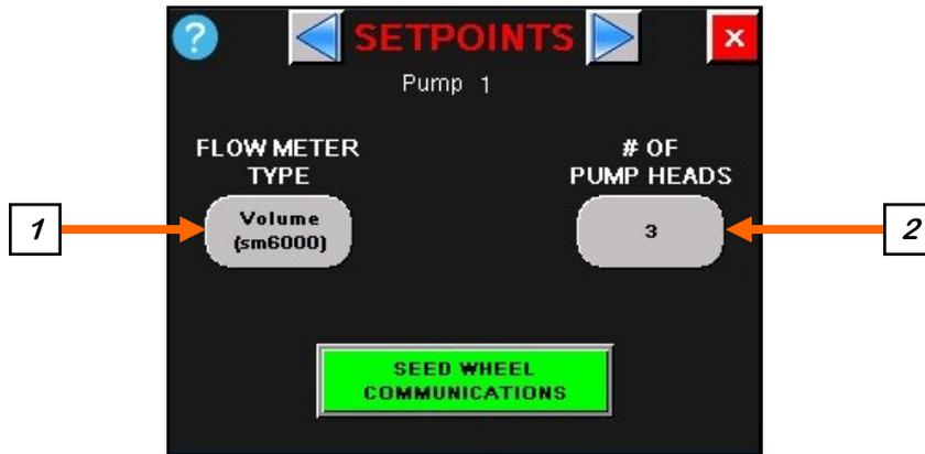
**1. FLOW METER TYPE:** Pressing this button toggles between Volumetric, Mass, Low Flow and the Custom flow meter options to match the type of flow meter being used with your equipment. If using a Non-USC type pump, it would be set to custom activating the Custom PID Settings button (see page 40).
