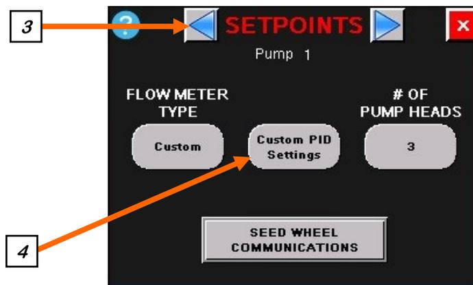
**3. ARROWS:** Selecting the arrow buttons allows the operator to scroll through all of the pumps to setup each one individually.
