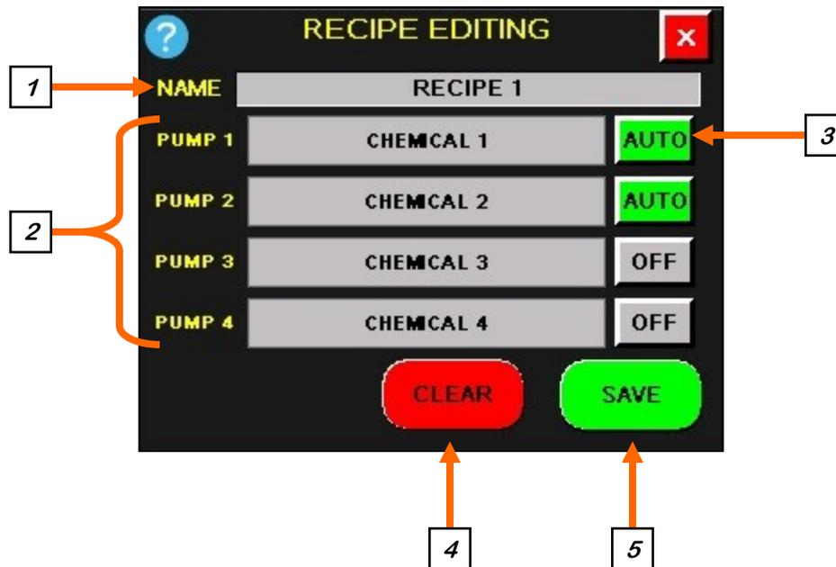
**1. RECIPE NAME:** When this button is pushed an alpha numeric keypad appears allowing the operator to create or change the recipe name.
