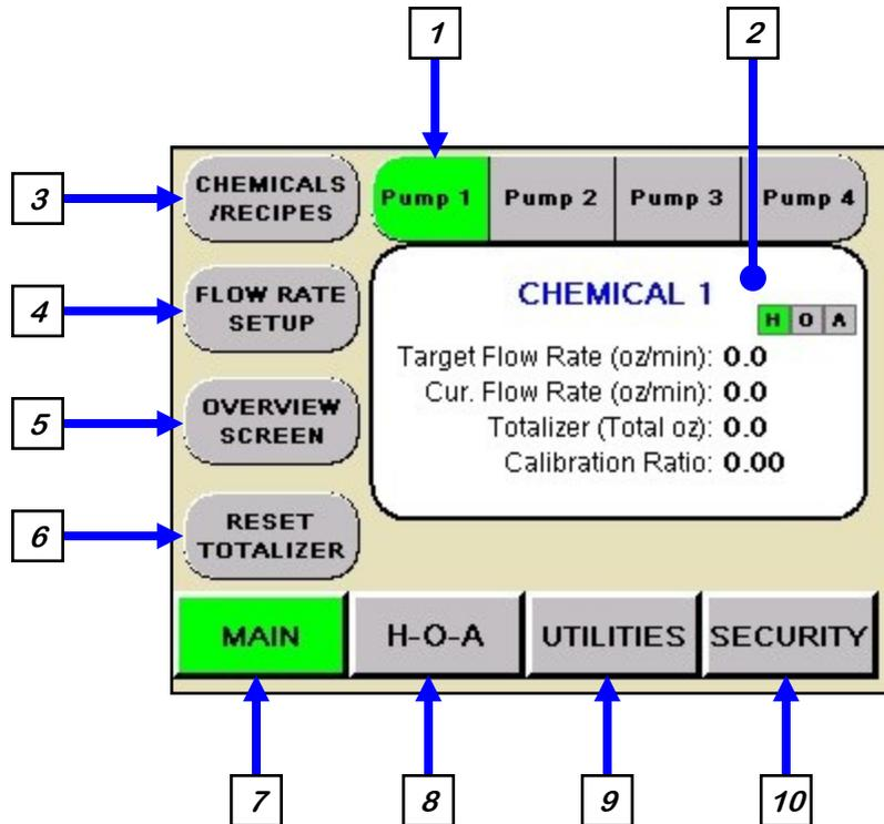
**1. PUMP IDENTIFICATION:** Displays which pump stand main screen the operator is in by highlighting it in green. It also allows the operator to move from one pump stand to another without returning to the Overview screen.
