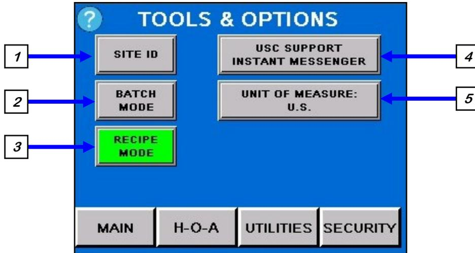
**1. SITE ID:** Pressing this button brings up the Site Identification screen. Press the Site Name field and an alpha numeric keyboard will appear for entering the name of the installation. The Site Description is automatically populated with the description of the current software loaded. This information will be used by USC service personnel to verify the customers installation.
