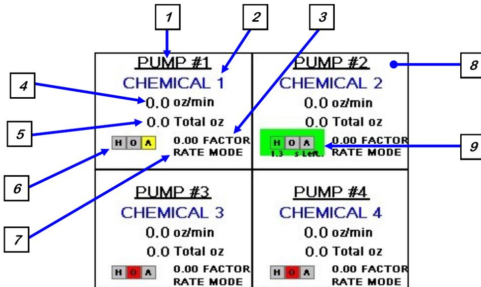
**1. PUMP IDENTIFICATION:** Displays the number of each individual pump controlled by the system.
