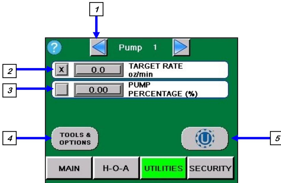
**1. ARROWS:** Selecting the arrow buttons allows the operator to scroll through all of the pumps to set up each one individually.
