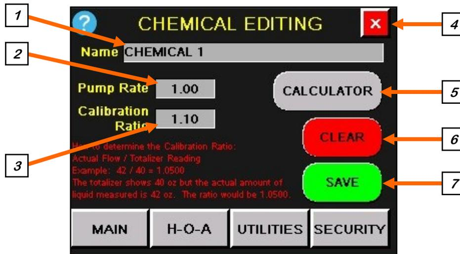
**1. CHEMICAL NAME:** When this button is pushed an alpha numeric keypad appears allowing the operator to change an existing chemical name. If an unused box was selected from the list, the name will be blank and the Calibration Ratio will be 1.0. allowing the operator to enter a new chemical into the system. Once saved, it will be added to the list.
