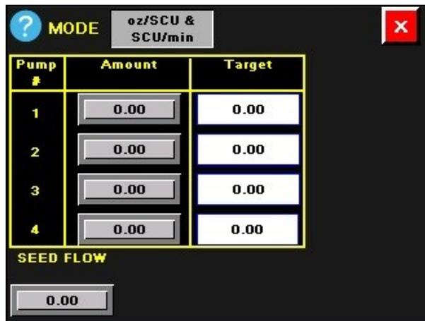
**MODE: oz / SCU & lb / min** - Allows the operator to enter the Seeds / Unit and Seed Count boxes as well as enter the treater seed flow in lb / min and the chemical application in oz / SCU. The system will convert it to oz / min and display it in the white box.
