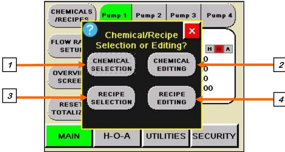
**1. CHEMICAL SELECTION:** Press this button and the Chemical Selection screen appears. (Bottom left) Use the arrows to scroll through the list to find the chemical you wish to use. The system can store up to 100 different chemical entries. Each chemical type will have its own name and calibration ratio. When operating in the Recipe mode, this button will become inactive because the recipe is now dictating the chemical selection.
