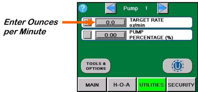
**FLOW METER CALIBRATION (USC Pump Stands)**
