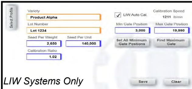
Checking the LIW Auto Cal. box will automatically calibrate the LIW Actuator during a run.
