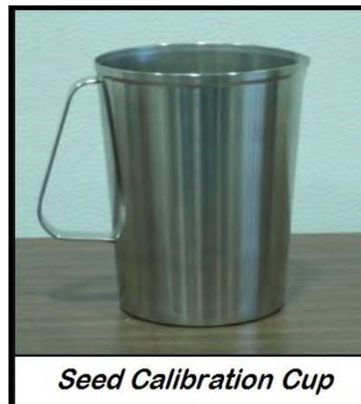
5. After the cup has been filled, strike off the top of the calibration cup with a straight edge (see page 33, figure 2).
