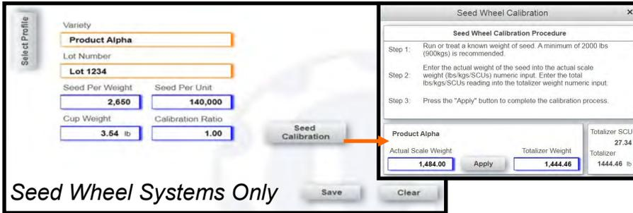
Pressing Seed Calibration causes a pop up screen to appear that allows for the calibration of the seed variety for the Seed Wheel.
