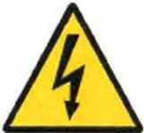
**International Electrocution Hazard.** This symbol indicates that an electrocution hazard exists. Serious injury or death could result from contacting high voltage.
