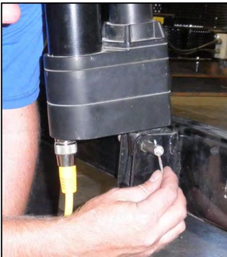
**STEP F:** Insert a cotter pin (06-09-0087) in the clevis pins at both ends of the actuator. Then, attach the yellow cable to the motor connector
