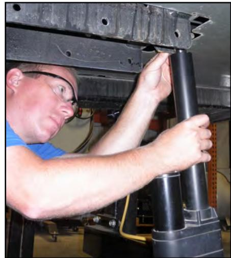
**STEP F:** Insert a cotter pin (06-09-0087) in the clevis pins at both ends of the actuator. Then, attach the yellow cable to the motor connector
