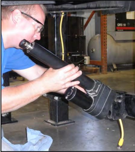
**STEP E:** Insert the second clevis pin (06-09-0058) and the two flat washers (06-05-0005) attaching the end of the actuator piston to the bracket on the drum frame. The washers should be on the outside of the frame bracket.
