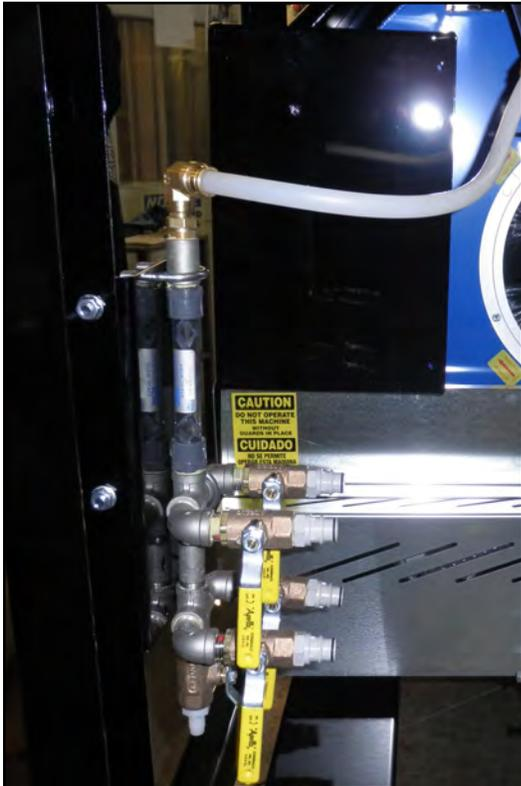
7. For LPV and LPX treaters, attach the chemical tubing from the pump stand(s) to the static mixer assembly plumbing on the seed treater (left). For all other treaters additional tubing may be added or removed to accommodate your set-up.
