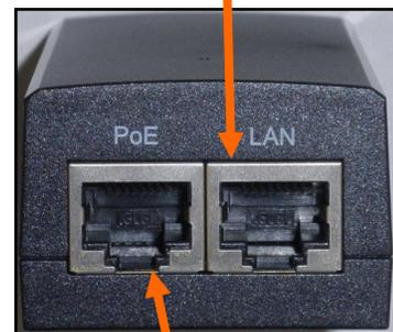
**STEP 4:** Slide the bottom cover off of the EAP. Plug one end of the other Ethernet cable to the PoE port on the power adapter and the other end to the Ethernet port on the bottom of the EAP unit. The EAP unit is pre-programmed to communicate with the control panel.
