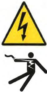
Electrocution accidents are most likely to occur during maintenance of the electrical system or when working on or near exposed high voltage wiring. This hazard does not exist when the electrical power has been disconnected, properly locked, and tagged out.
