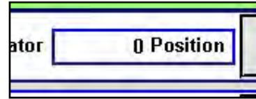
**2. LIW ACTUATOR PERCENT POSITION:** When this button is pressed, a numeric touch pad (right) will appear to allow the operator to manually adjust the percentage of the actuator gate. When running in the Auto mode the program will override this manual setting.
