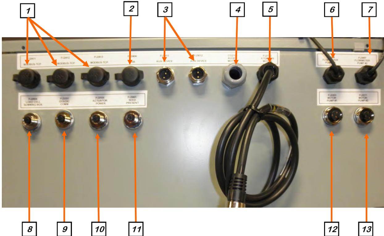
1. There are three MODBUS TCP Ethernet connectors on the Control Panel. These are used as a wireless access point for tablet control and U-Connect Pro to connect to the panel.
