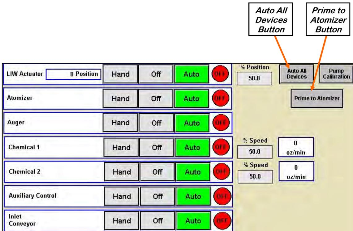
3. Return to the main screen and press the Start Setup button. Press the gray buttons to change the Recipe or Seed Type fields. Press Start to begin the run. The atomizer and auger will turn on. Open the manual gate on the box. When the proximity switch detects seed, a timer will count down the number of seconds the start delay was set for. When that time elapses, the slide gate will open.
