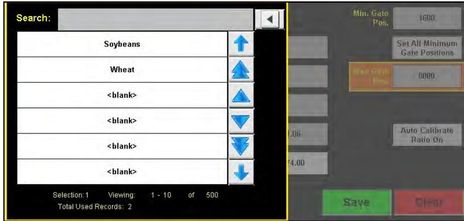
**1A. MINIMUM GATE POSITION:** Pressing this button brings up a keypad to enter a value for a minimum gate position for this individual seed profile.
