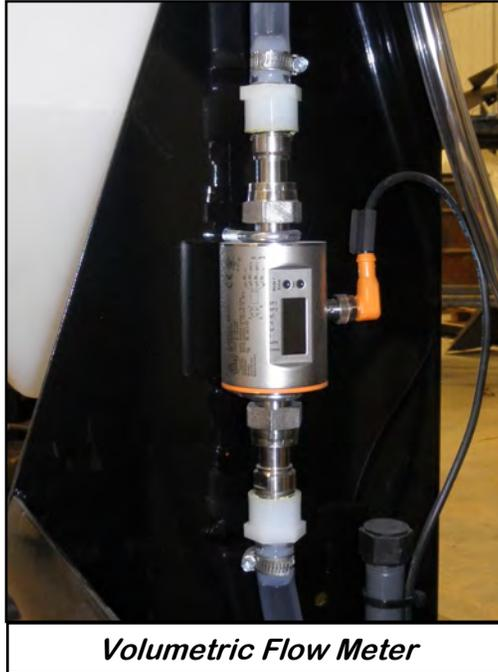
Proper calibration of the liquid system is critical to achieve a proper granular / chemical mixture. For information on pump calibration and flow meter calibration to determine liquid flow rate, see the Calibration and Operation section on page 48.
