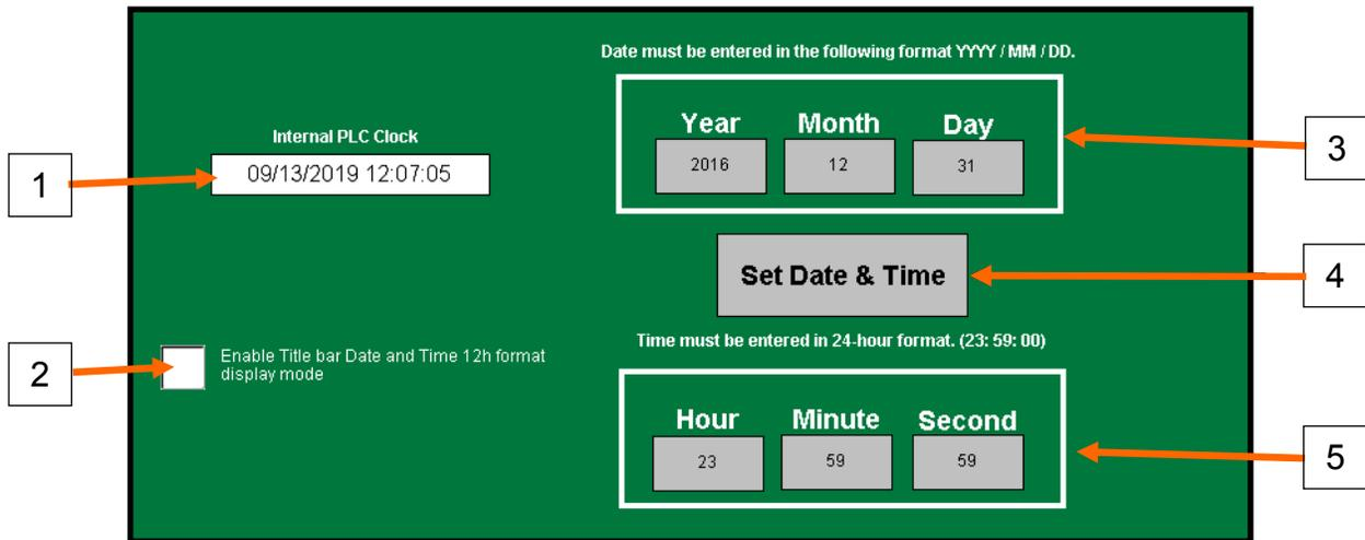
1. **Internal PLC Clock:** Displays the currently set time for the pump controller.
