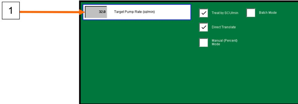
**1. Target Pump Rate:** Selecting the grey box allows the operator to enter the target pump rate by either oz/min or mL/min. This rate is independent of any treater or seed information and will strictly try and achieve the requested flow rate. This option appears when the “Direct Translate” check box is selected.
