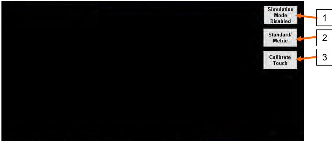
1. **Simulation Mode Button:** Turns on simulation of the pump stand panel. In simulation the pump will not start and the inputs will be simulated.
