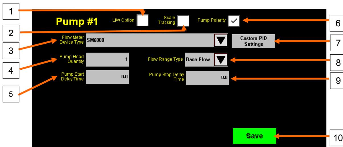
1. **LIW Option:** Selecting this option toggles the pump stand type between LIW and Flow Meter Type pump.
