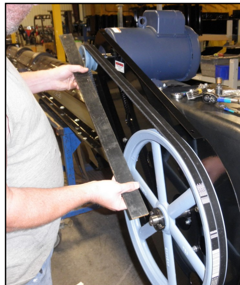
Lay a Straightedge Across Pulley Faces
